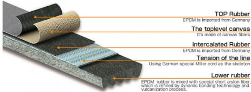
Single - sided Auxiliary drive belt,cross - section structure diagram
