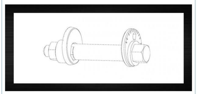
If the wheel camber is outside the standard range of use, it can only be adjusted by using eccentric bolts, which ensure that the wheel data is normal and prevent wheel wear.
