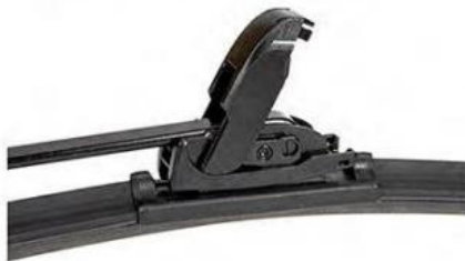
3 Insert arm into the adaptor interface
