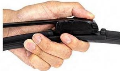
4 Clamp the cap, installation is complete
