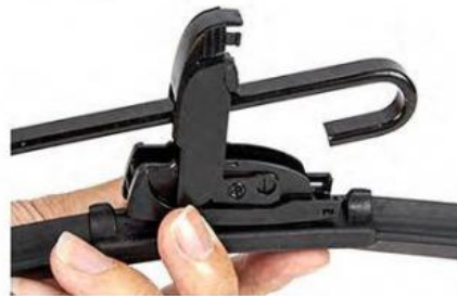
2 push wiper arm through adapter cap
