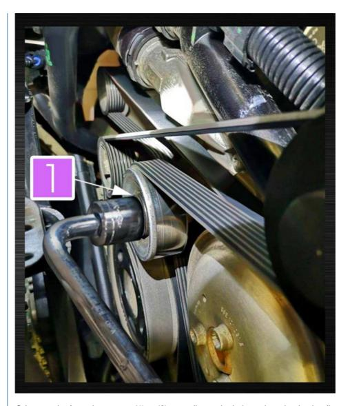
⑤ Loosen the fastening screws (1) or (2) according to the belt tension wheel to be dismounted.
