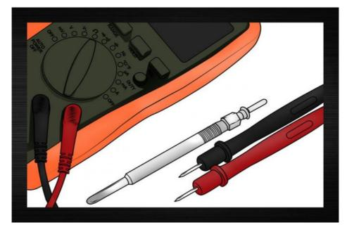
Normally, if the glow plug is broken, the electric heating indicator on the dashboard will be on all the time, or in low temperature weather, the engine is difficult to start, which may also be the failure of the preheating system. The glow plug is an important accessory of the ignition system of the car.
